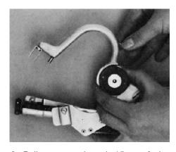
**3.** Pull out approximately 15 cm of wire and thread it through the wire guide and nozzle.
