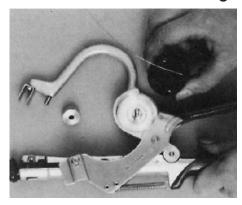
**1.** Slacken knurled nut and remove old reel.
