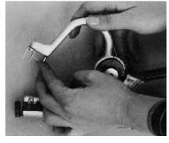
**4.** Bend approximately 1 cm of the end of the wire upwards in the direction of the press-in device.
