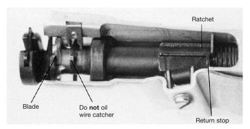
There must always be a light film of oil in the area of the blade and between the return stop and ratchet. Oil these areas as necessary.
