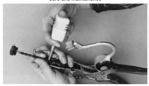
The helix should always be covered with a light film of oil. Withdraw the helix to oil.
