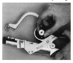
**5.** Close the tool until the wire is held. Turn the knurled nut counter-clockwise to slacken the reel brake until the tool opens on its own.
