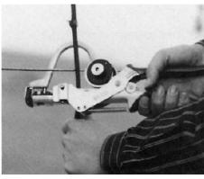
2. ... without using too much force close the tool until the wire is clamped in the aperture.
