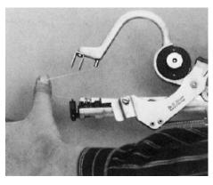
**6.** Use a thumb to form a loop in the wire and close the **tool without exerting too much force** until **a slight** click is heard.
