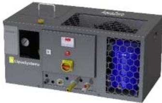
The small refrigerators are compact and easily connect to an existing pipeline system. They are equipped with a water tank and centrifugal pump. In outlet temperatures below + 10 ° C is the use of antifreeze (glycol, 34%) required.
