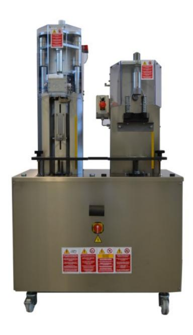
Manual monoblock provides both corking and wire-hooding in a single machine. It can be used for bottling in glass
