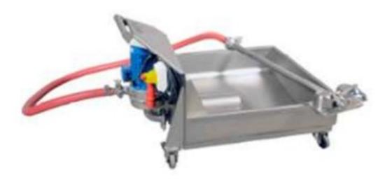
A bathtub, a tank on wheels, equipped with a fancy pump for washing tanks with various types of cleaning solutions. Made entirely of Aisi 304 stainless steel, a pump with a double stainless steel turbine, a pre-filter at the pump entrance, a connecting pipe and a washing nozzle with a Teflon base. The device is intended for washing tanks with a maximum height of 3 meters.
